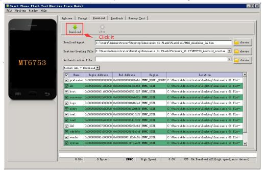
2) Next, turn off G1 player and connect it to your computer with the supplied USB-C cable. The update tool will automatically recognize the connected device and start formatting and updating the firmware. You can see the percentage of completion through the color progress bar below, until 100% complete.
